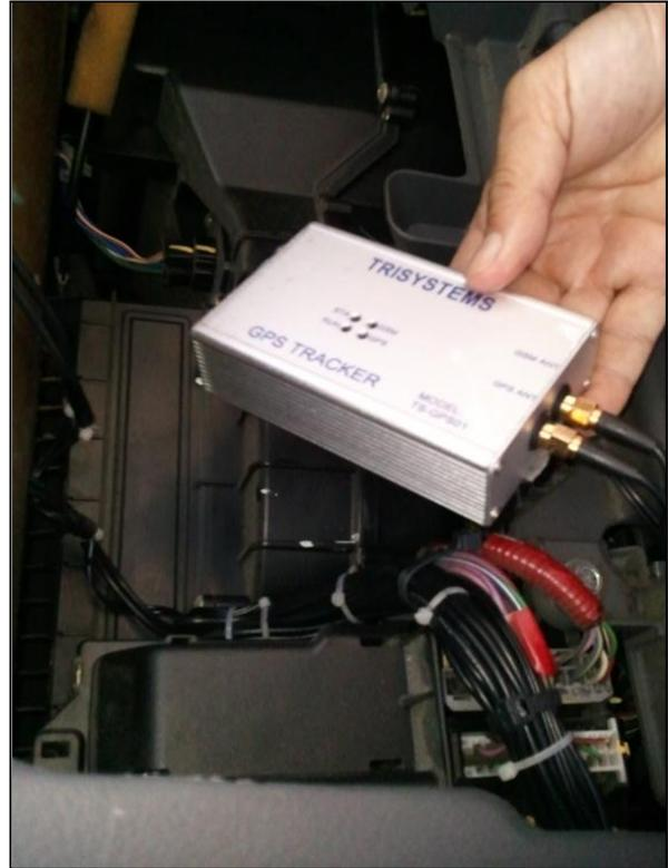
**Connecting Cables to the GPS Tag**
